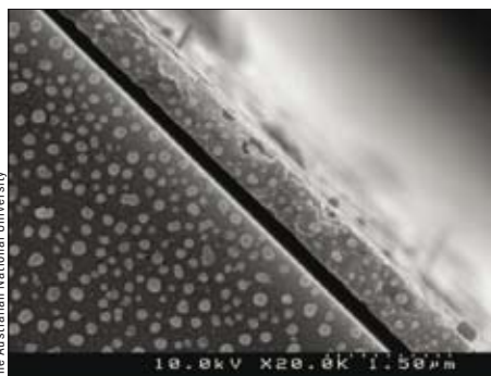
A SEM image of silver nanoparticles on a solar cell, each averaging only 100 nm in diameter.
