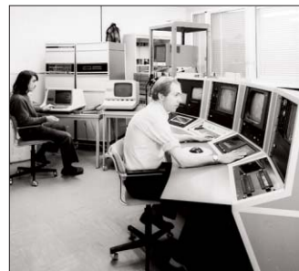
The prototype SPS control desk is shown under test with the NORD-10 computer (December 1973).
